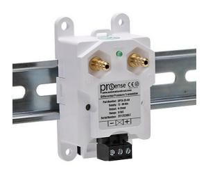
ProSense air differential pressure transmitter, 0 to 3.0in of water column range, 4-20 mA analog output, 1/4in brass barbed process connection, 12 to 36 VDC operating voltage, screw terminals, 35mm DIN rail or panel mount.
