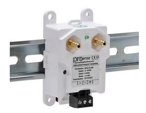
ProSense air differential pressure transmitter, -3.0 to +3.0in of water column range, 4-20 mA analog output, 1/4in brass barbed process connection, 12 to 36 VDC operating voltage, screw terminals, 35mm DIN rail or panel mount.
