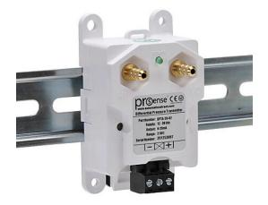
ProSense air differential pressure transmitter, 0 to 2.0in of water column range, 4-20 mA analog output, 1/4in brass barbed process connection, 12 to 36 VDC operating voltage, screw terminals, 35mm DIN rail or panel mount.
