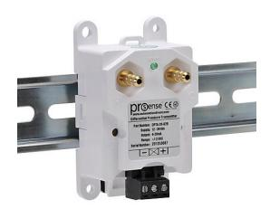
ProSense air differential pressure transmitter, -2.0 to +2.0in of water column range, 4-20 mA analog output, 1/4in brass barbed process connection, 12 to 36 VDC operating voltage, screw terminals, 35mm DIN rail or panel mount.
