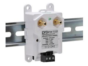
ProSense air differential pressure transmitter, -2.0 to +2.0in of water column range, 4-20 mA analog output, 1/4in brass barbed process connection, 12 to 36 VDC operating voltage, screw terminals, 35mm DIN rail or panel mount.
