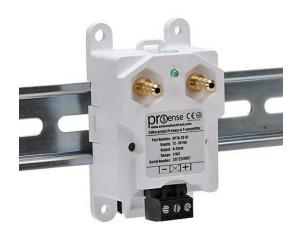
ProSense air differential pressure transmitter, 0 to 1.0in of water column range, 4-20 mA analog output, 1/4in brass barbed process connection, 12 to 36 VDC operating voltage, screw terminals, 35mm DIN rail or panel mount.
