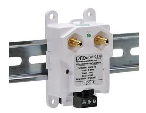
ProSense air differential pressure transmitter, -1.0 to +1.0in of water column range, 4-20 mA analog output, 1/4in brass barbed process connection, 12 to 36 VDC operating voltage, screw terminals, 35mm DIN rail or panel mount.
