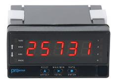
ProSense digital panel meter, panel mount, 1/8 DIN, 14mm 5-digit tri-color (red, green, amber) LED, pulse or frequency input, 85-265 VAC/100-300 VDC operating voltage.
