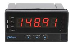
ProSense digital panel meter, panel mount, 1/8 DIN, 14mm 5-digit tri-color (red, green, amber) LED, analog, load cell, RTD or thermocouple input, 22-53 VAC/10.5-70 VDC operating voltage.
