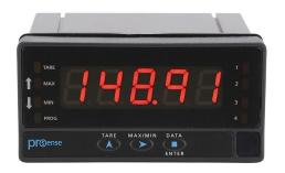
ProSense digital panel meter, panel mount, 1/8 DIN, 14mm 5-digit tri-color (red, green, amber) LED, analog, load cell, RTD or thermocouple input, 85-265 VAC/100-300 VDC operating voltage.
