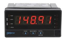
ProSense digital panel meter, panel mount, 1/8 DIN, 14mm 5-digit tri-color (red, green, amber) LED, analog, load cell, RTD or thermocouple input, 4-20 mA output, 22-53 VAC/10.5-70 VDC operating voltage.
