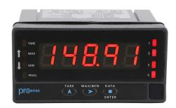
ProSense digital panel meter, panel mount, 1/8 DIN, 14mm 5-digit tri-color (red, green, amber) LED, analog, load cell, RTD or thermocouple input, (4) 5A SPST relays output, 22-53 VAC/10.5-70 VDC operating voltage.
