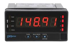
ProSense digital panel meter, 1/8 DIN, 14mm 5-digit tri-color (red, green, amber) LED, analog, RTD or thermocouple input, (4) 5A SPST relays output, 22 to 53 VAC/10.5 to 70 VDC operating voltage.
