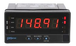
ProSense digital panel meter, panel mount, 1/8 DIN, 14mm 5-digit tri-color (red, green, amber) LED, analog, load cell, RTD or thermocouple input, (2) 8A SPDT relays output, 22-53 VAC/10.5-70 VDC operating voltage.
