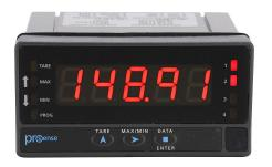
ProSense digital panel meter, panel mount, 1/8 DIN, 14mm 5-digit tri-color (red, green, amber) LED, analog, load cell, RTD or thermocouple input, (2) 8A SPDT relays output, 85-265 VAC/100-300 VDC operating voltage.
