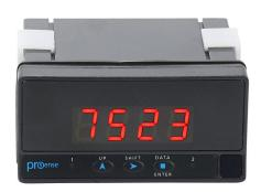
ProSense digital panel meter, panel mount, 1/8 DIN, 14mm 4-digit red LED, pulse or frequency input, 20-265 VAC/11-265 VDC operating voltage.
