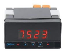
ProSense digital panel meter, 1/8 DIN, 14mm 4-digit red LED, pulse and frequency input, (2) 8A SPDT relays output, 20 to 265 VAC/11 to 265 VDC operating voltage.
