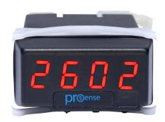
ProSense digital panel meter, panel mount, 1/32 DIN, 10mm 4-digit red LED, pulse or frequency input, 21-53 VAC/10.5-70 VDC operating voltage.
