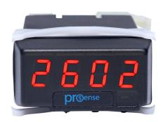
ProSense digital panel meter, panel mount, 1/32 DIN, 10mm 4-digit red LED, pulse or frequency input, 85-265 VAC/100-300 VDC operating voltage.
