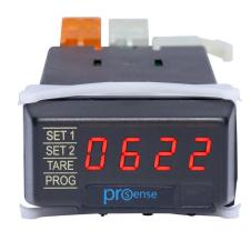
ProSense digital panel meter, panel mount, 1/32 DIN, 8mm 4-digit red LED, pulse or frequency input, 0/4-20 mA or (2) 5A SPST relays output, 21 to 53 VAC/13.5 to 70 VDC operating voltage.
