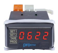
ProSense digital panel meter, panel mount, 1/32 DIN, 8mm 4-digit red LED, pulse or frequency input, 0/4-20 mA or (2) 5A SPST relays output, 21-53 VAC/13.5-70 VDC operating voltage.
