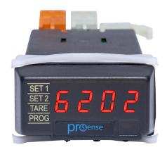
ProSense digital panel meter, panel mount, 1/32 DIN, 8mm 4-digit red LED, pulse or frequency input, 0/4-20 mA or (2) 5A SPST relays output, 85-265 VAC/100-300 VDC operating voltage.
