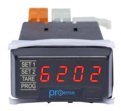
ProSense digital panel meter, 1/32 DIN, 8mm 4-digit red LED, pulse and frequency input, 0/4-20 mA and (2) 5A SPST relays output, 85 to 265 VAC/100 to 300 VDC operating voltage.
