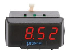
ProSense digital panel meter, panel mount, 1/32 DIN, 10mm 4-digit red LED, analog input, loop powered.
