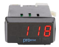
ProSense digital panel meter, panel mount, 1/32 DIN, 10mm 4-digit red LED, analog input, 85-265 VAC/100-300 VDC operating voltage.
