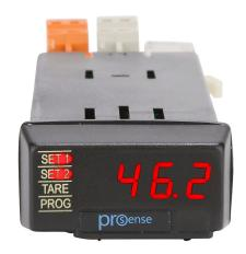
ProSense digital panel meter, panel mount, 1/32 DIN, 8mm 4-digit red LED, analog input, (2) 5A SPST relays output, 21-53 VAC/10.5-70 VDC operating voltage.
