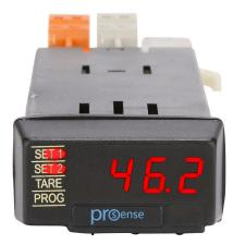
ProSense digital panel meter, panel mount, 1/32 DIN, 8mm 4-digit red LED, analog input, (2) 5A SPST relays output, 85-265 VAC/100-300 VDC operating voltage.
