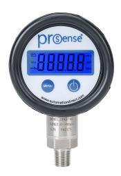
ProSense digital pressure gauge, 0 to 60 psig, 0.5% of full scale accuracy, stainless steel wetted parts, 1/4in male NPT process connection, lower mount.
