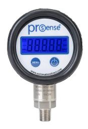
ProSense digital pressure gauge, 0 to 600 psig, 0.5% of full scale accuracy, stainless steel wetted parts, 1/4in male NPT process connection, lower mount.
