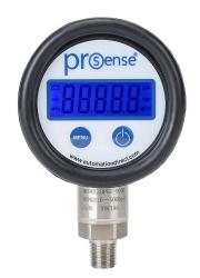
ProSense digital pressure gauge, 0 to 5000 psig, 0.5% of full scale accuracy, stainless steel wetted parts, 1/4in male NPT process connection, lower mount.
