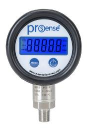
ProSense digital pressure gauge, 0 to 30 psig, 0.5% of full scale accuracy, stainless steel wetted parts, 1/4in male NPT process connection, lower mount.
