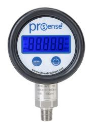
ProSense digital pressure gauge, 0 to 300 psig, 0.5% of full scale accuracy, stainless steel wetted parts, 1/4in male NPT process connection, lower mount.
