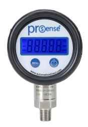
ProSense digital pressure gauge, 0 to 200 psig, 0.5% of full scale accuracy, stainless steel wetted parts, 1/4in male NPT process connection, lower mount.
