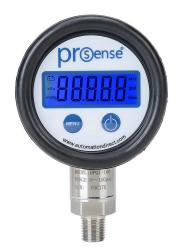
ProSense digital pressure gauge, 0 to 100 psig, 0.5% of full scale accuracy, stainless steel wetted parts, 1/4in male NPT process connection, lower mount.
