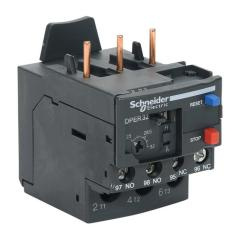
Schneider Electric Easy TeSys series thermal overload relay, 23-32A adjustable, bi-metallic, direct mount power connection(s). For use with Schneider Electric DPE09 to DPE38 contactors.
