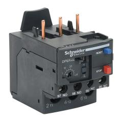
Schneider Electric Easy TeSys series thermal overload relay, 16-24A adjustable, bi-metallic, direct mount power connection(s). For use with Schneider Electric DPE09 to DPE38 contactors.
