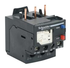
Schneider Electric Easy TeSys series thermal overload relay, 9-13A adjustable, bi-metallic, direct mount power connection(s). For use with Schneider Electric DPE09 to DPE38 contactors.
