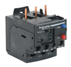
Schneider Electric Easy TeSys series thermal overload relay, 7-10A adjustable, bi-metallic, direct mount power connection(s). For use with Schneider Electric DPE09 to DPE38 contactors.
