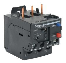
Schneider Electric Easy TeSys series thermal overload relay, 5.5-8A adjustable, bi-metallic, direct mount power connection(s). For use with Schneider Electric DPE09 to DPE38 contactors.
