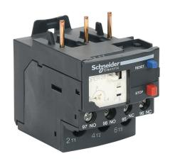
Schneider Electric Easy TeSys series thermal overload relay, 2.5-4A adjustable, bi-metallic, direct mount power connection(s). For use with Schneider Electric DPE09 to DPE38 contactors.
