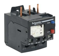
Schneider Electric Easy TeSys series thermal overload relay, 1-1.6A adjustable, bi-metallic, direct mount power connection(s). For use with Schneider Electric DPE09 to DPE38 contactors.
