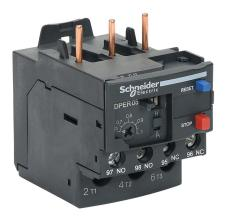
Schneider Electric Easy TeSys series thermal overload relay, 0.63-1A adjustable, bi-metallic, direct mount power connection(s). For use with Schneider Electric DPE09 to DPE38 contactors.
