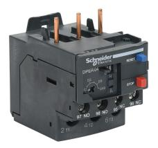
Schneider Electric Easy TeSys series thermal overload relay, 0.40-0.63A adjustable, bi-metallic, direct mount power connection(s). For use with Schneider Electric DPE09 to DPE38 contactors.
