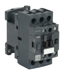
Schneider Electric Easy TeSys series IEC contactor, 38A, (3) N.O. power poles, (1) N.O. auxiliary contacts, 120 VAC (50/60Hz) coil voltage.
