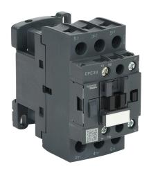
Schneider Electric Easy TeSys series IEC contactor, 38A, (3) N.O. power poles, (1) N.O. auxiliary contacts, 24 VAC (50/60Hz) coil voltage.
