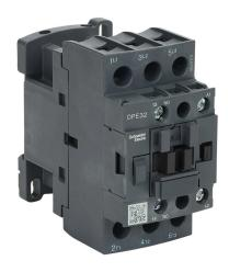
Schneider Electric Easy TeSys series IEC contactor, 32A, (3) N.O. power poles, (1) N.O. auxiliary contacts, 240 VAC (50/60Hz) coil voltage.
