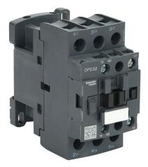
Schneider Electric Easy TeSys series IEC contactor, 32A, (3) N.O. power poles, (1) N.O. auxiliary contacts, 120 VAC (50/60Hz) coil voltage.
