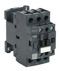
Schneider Electric Easy TeSys series IEC contactor, 32A, (3) N.O. power poles, (1) N.O. auxiliary contacts, 24 VAC (50/60Hz) coil voltage.
