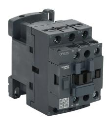
Schneider Electric Easy TeSys series IEC contactor, 25A, (3) N.O. power poles, (1) N.O. auxiliary contacts, 120 VAC (50/60Hz) coil voltage.
