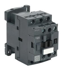
Schneider Electric Easy TeSys series IEC contactor, 25A, (3) N.O. power poles, (1) N.O. auxiliary contacts, 24 VAC (50/60Hz) coil voltage.
