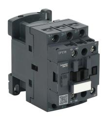
Schneider Electric Easy TeSys series IEC contactor, 18A, (3) N.O. power poles, (1) N.O. auxiliary contacts, 240 VAC (50/60Hz) coil voltage.
