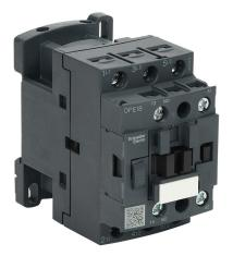
Schneider Electric Easy TeSys series IEC contactor, 18A, (3) N.O. power poles, (1) N.O. auxiliary contacts, 120 VAC (50/60Hz) coil voltage.
