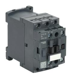
Schneider Electric Easy TeSys series IEC contactor, 18A, (3) N.O. power poles, (1) N.O. auxiliary contacts, 24 VDC coil voltage.
