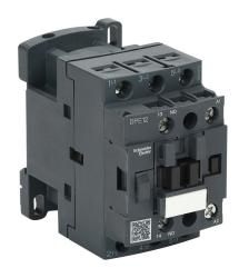
Schneider Electric Easy TeSys series IEC contactor, 12A, (3) N.O. power poles, (1) N.O. auxiliary contacts, 240 VAC (50/60Hz) coil voltage.
